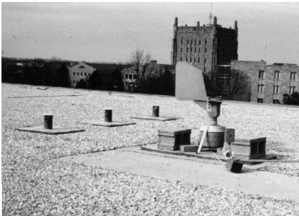
Fig. 2. Sampling Site on the roof of Oliphant Hall at The University of Tulsa with the Burkard Spore Trap on the right and three Tauber traps on the left.
