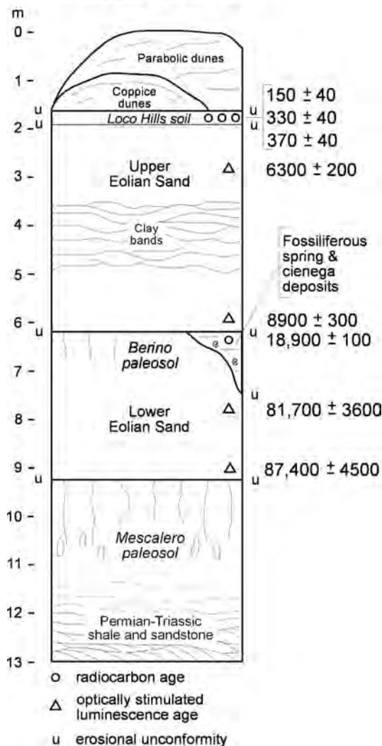
Figure 1. Composite stratigraphy and age of the Mescalero Sands, southeastern New Mexico; no single exposure incorporates all stratigraphic units together.
